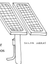
Most solar systems today add a device called an inverter that converts DC battery power to more conventional 120 Volt AC power that 99% of American appliances use. By using this type of set-up you can run a normal household on solar electricity without any basic changes in wiring of the house.
