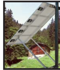
Series 4002 with SolarMount® standard rails for 2.5" (65 mm) Schedule 40 or 80 steel pole, outside dia. 2.875" (73.0 mm); 3" (80 mm) Schedule 40 or 80 steel pole, outside dia. 3.500" (88.9 mm); or 4" (100 mm) Schedule 40 or 80 steel pole, outside dia. 4.500" (114.3 mm)
