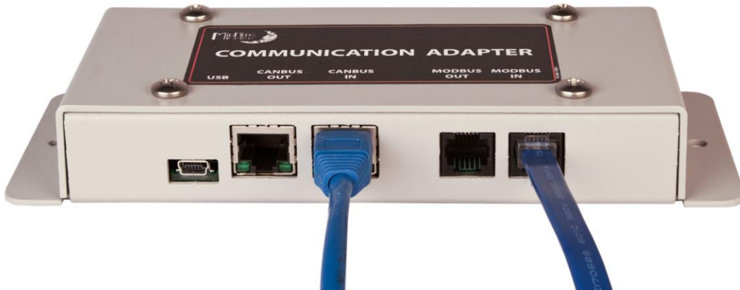
Typical Wall Mounted Connections
