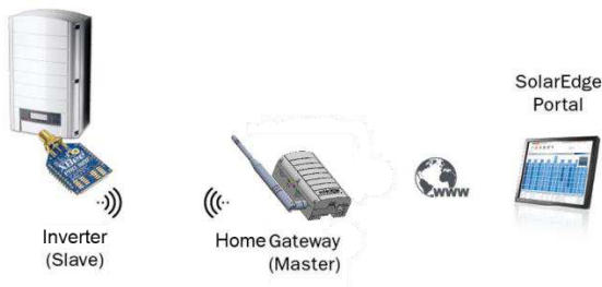
Figure 2: Connection to the SolarEdge Inverter
